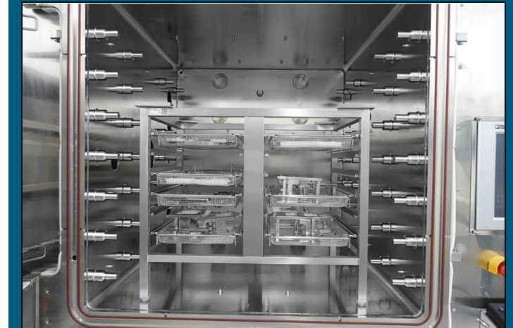
Vacuum chamber (vacuum pressure adjustable) Environment Class 1 cleanroom (ISO 14644-1)
