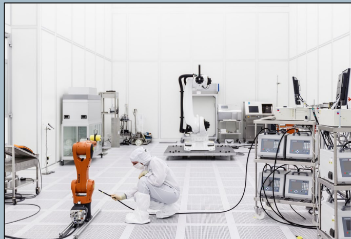
Class 1 clean room (ISO 14644-1) with relative humidity 45 %
