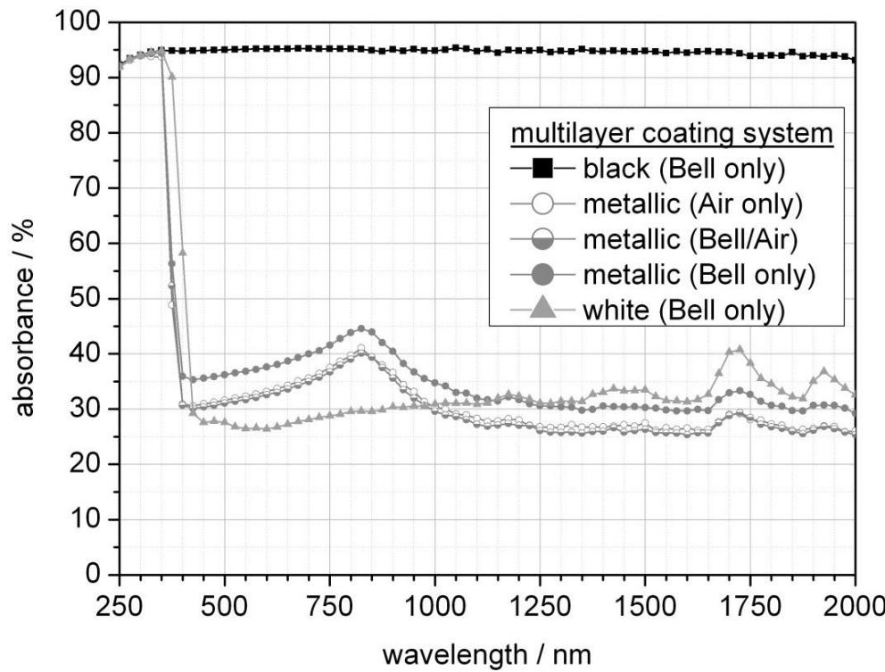
Whereas the white coating showed a low absorption in the wavelength range between 250 and 1000 nm, the absorption of the black system was very high, with values above 90 %. The metallic coating system, in comparison to the white coating, showed a slightly increased absorption, dependent on the kind of spray application.
