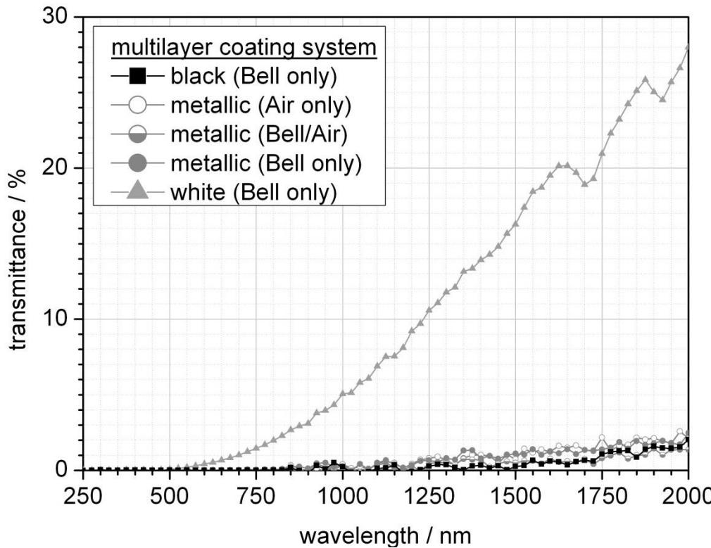
Because the observed transmittance is very small, the UV transparency of overcoated layers cannot be the only parameter, which influences the photooxidative degradation of the e-coat.
