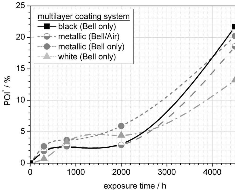
After 4500 h of WOM exposure, the following ranking of changes in POI was observed (ordered from higher to lower degradation):
