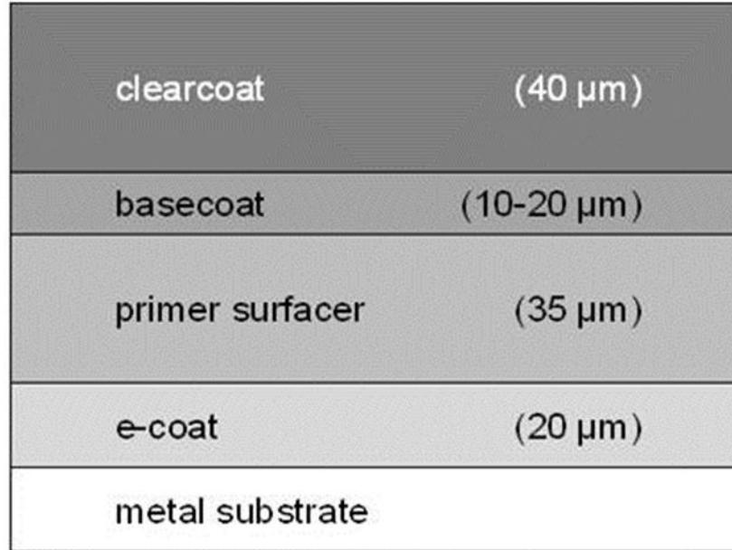
Todays automotive multilayer systems consist of an e-coat (mostly a cataphoretic coating), followed by a primer surfacer, a basecoat and a final clearcoat layer on the top.
