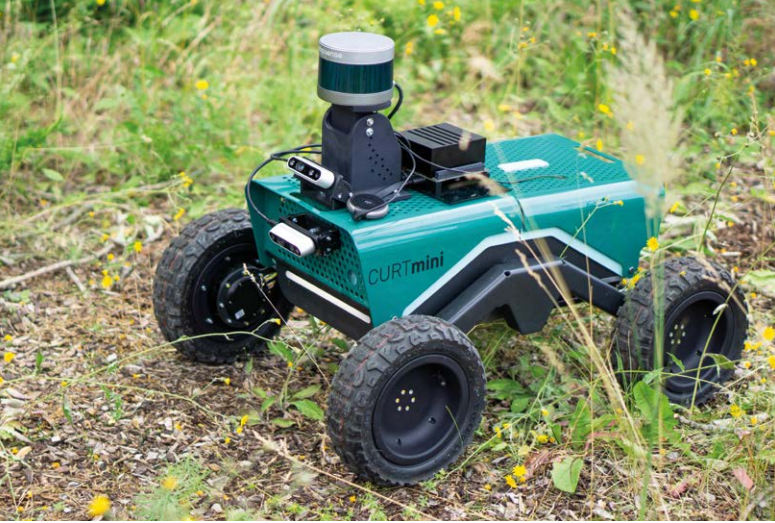
Mobile robot for various areas of application, including inspection tasks: CURTmini.
