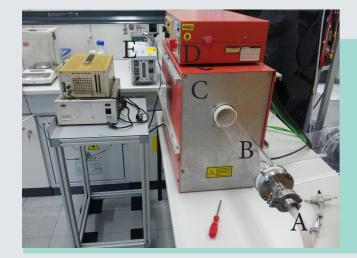
Supply for formic gas D = Temperature controller E = PumpQuartz tube = Reactor
