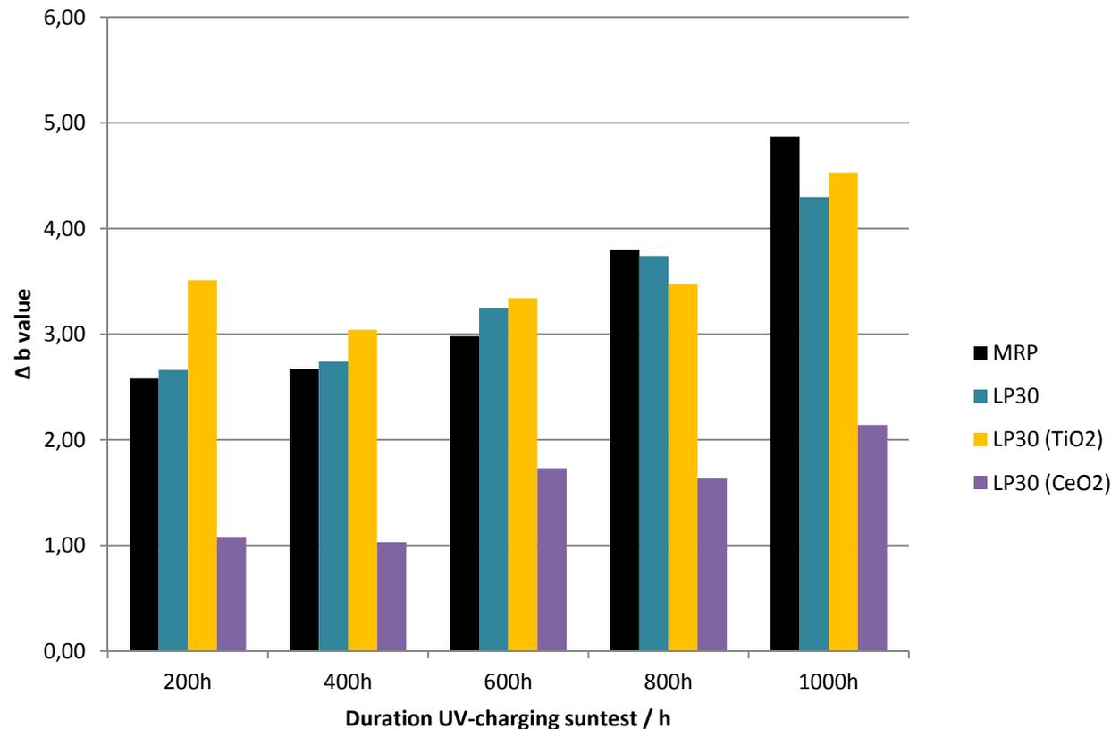
⇒ For the **nanoscale talcum LP30 treated with Ce-oxide**, in the more transparent primer with reduced pigment concentration, **improved UV-protection properties** were obtained, in comparison to the reference systems which contains (MRP, MLP) or doesn't contain TiO<sub>2</sub> (MLPa) pigments
