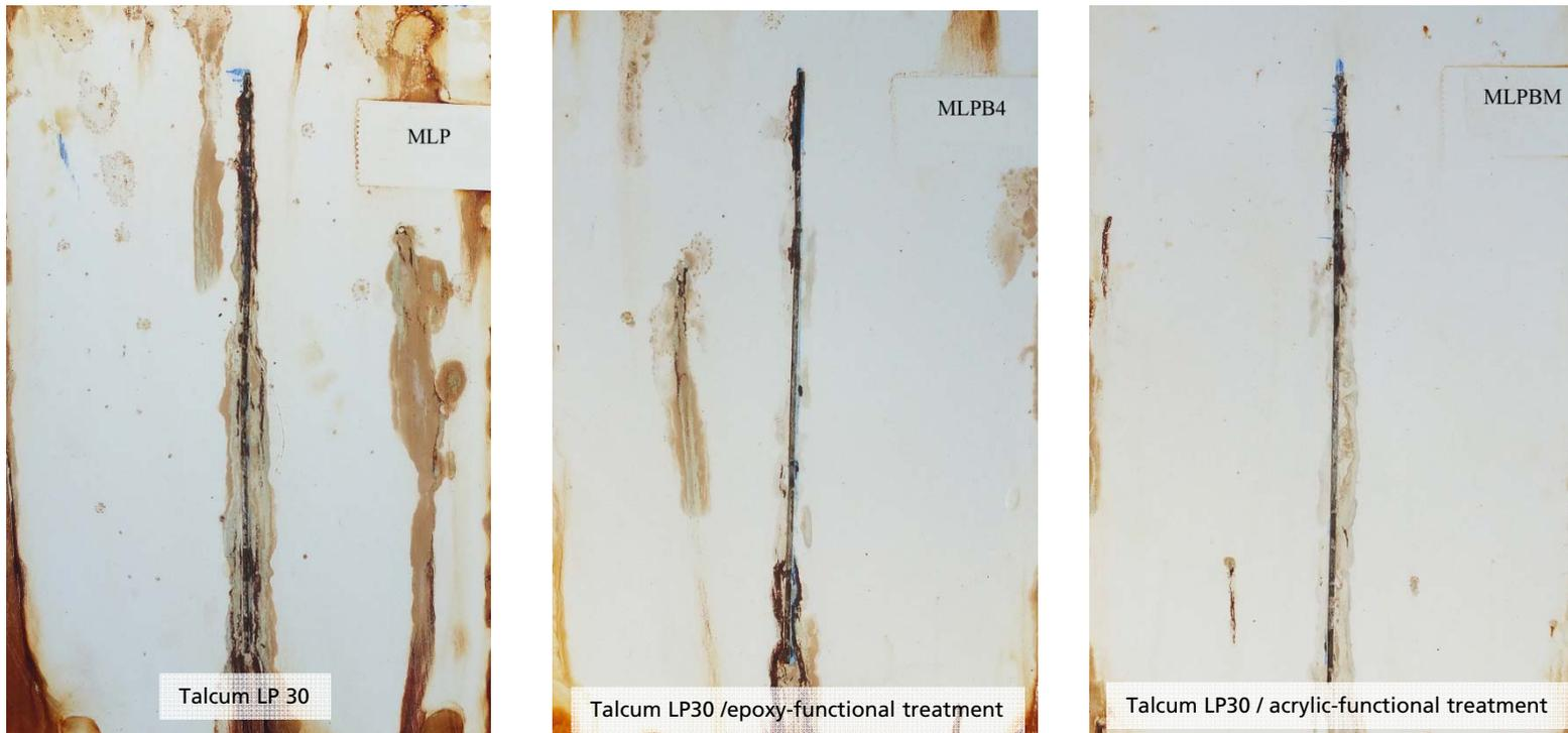
⇒ For the nanoscale talcum LP30 with different organic treatment excellent barrier and corrosion protection was observed
