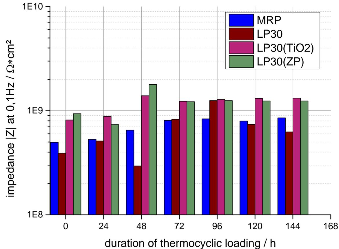
⇒ The improved corrosion protection of the nanoscale talcum modified with Zn-phosphate (ZP) could also be confirmed by performing impedance measurements
