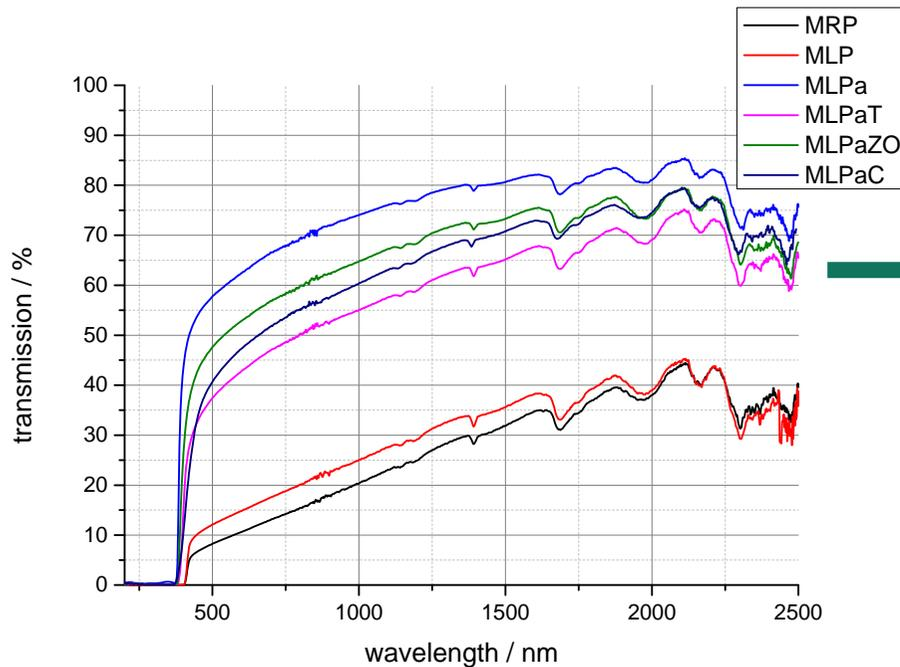
For primer coatings without  $\text{TiO}_2$ , containing inorganically modified nanoscale talcum LP30, higher transparency values from 500 nm to 2500 nm were obtained
