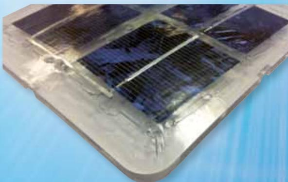
*Overmolded photovoltaic cells with polycarbonate*
