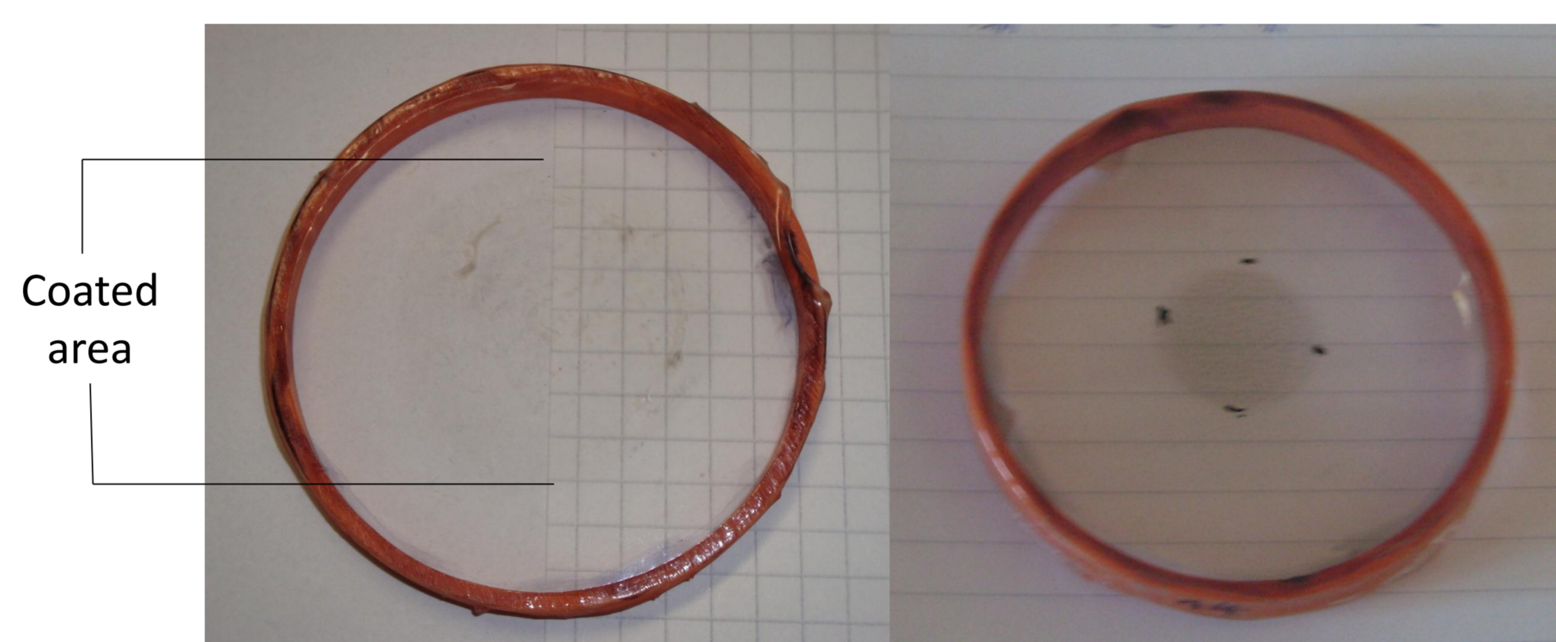
Fig. 4 CNT film deposited on elastomer substrate: (left) by spray coating; (right) by inkjet printing
