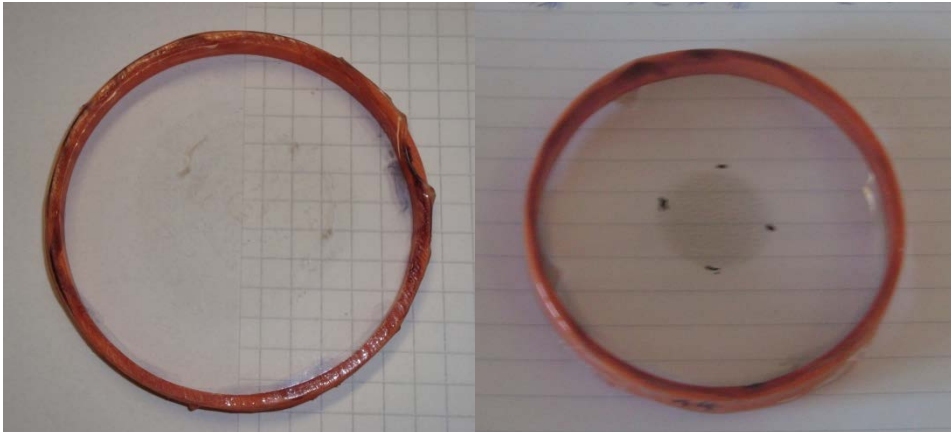
CNT film deposited on elastomer substrate: (left) by spray coating; (right) by inkjet printing
