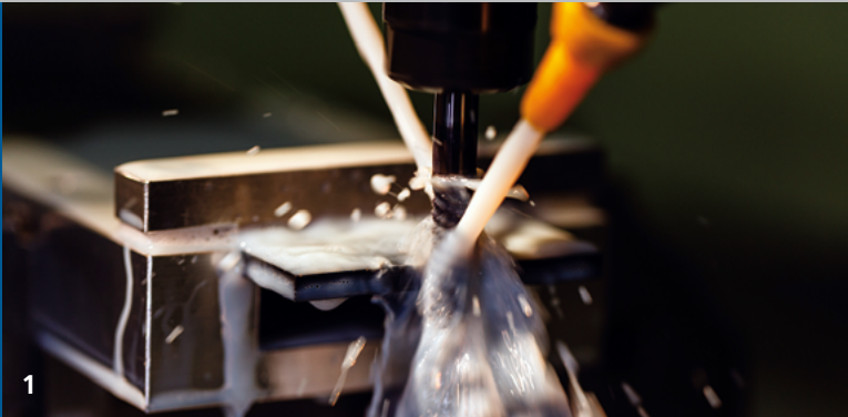
1 Machining of carbon fiber reinforced plastic (CFRP) workpiece with application of cutting fluid.
