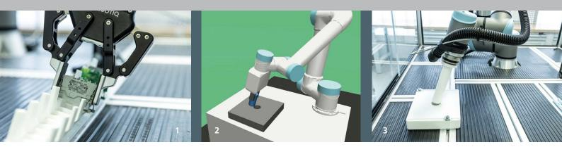
Robot picking up a control cabinet terminal for assembly.
