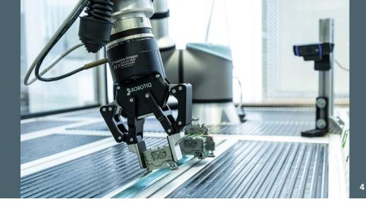
implemented in the framework control the robot so that it learns the underlying assembly process in the simulation through trial and error – without using or possibly damaging a single, real component. Artificial intelligence takes over the programming of the robot, even enabling the above-mentioned control cabinets to be assembled.
