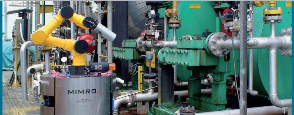
1 MIMROex during field testing on an offshore platform
