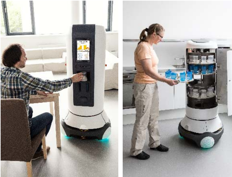
Figures: The robotic ServiceAssistant serving a drink, the robot is easy to fill with trays
