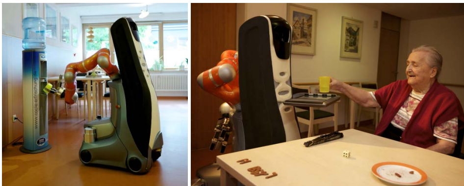
Figures: Care-O-bot fetching water from a water dispenser and offering it to a resident
