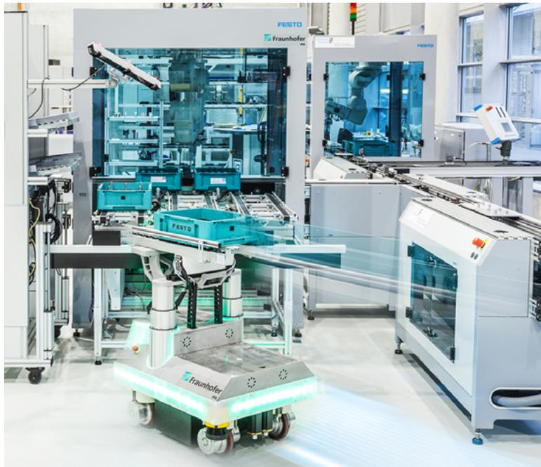
Automated guided vehicles can be located highly accurately with the aid of external sensors linked to the cloud. (Source: Fraunhofer IPA, photo: Rainer Bez)
