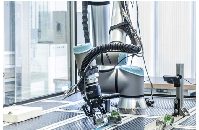
In the rob-aKademi research project, robots learn how to assemble so that more flexible programming is possible.
