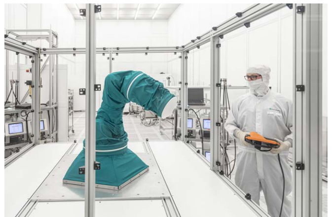
The patented 2ndSCIN® protective cover makes any moving automation components suitable for cleanrooms.
