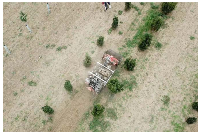
An agricultural robot from Fraunhofer IPA takes over weed control in a tree nursery.
